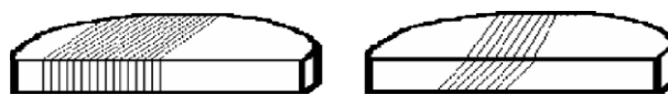
Fig. 1. A schematic representation of 90^{\circ} and 45^{\circ} microtome cuts of an ISDU aligned DPPC membrane.
